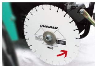
① Up-cut method for exceptionally effective cutting dust collection
