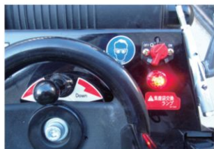
③ Warning LED lamp for dust collection bag change ※ 2
