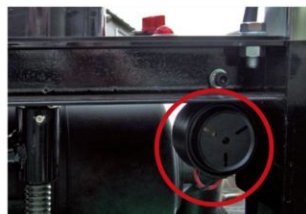
④ Warning buzzer for dust collection bag full ※ 2
